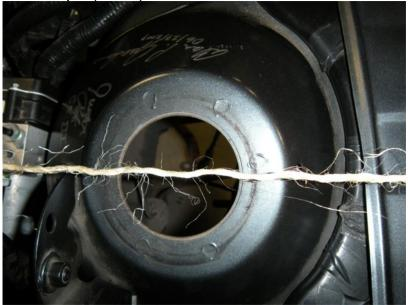
2. Using the string line as an approximate centre place the alloy mount over the strut top, aligning the adjusting slots in the plate with the string line. Make sure the mount is centred over the hole in the strut top (Pic 2)
