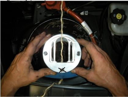
4. Use tape to hold the alloy mount in place while the mounting holes are marked with a centre punch. (Pic 4)
