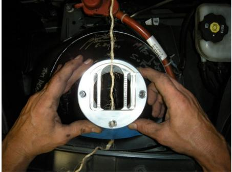
3. Make sure that the stud hole in the top mount that is in line with the adjusting slots and the string (marked with X) faces towards the outside (fender) of the engine bay (Pic 3)
