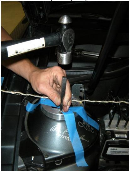
5. Using a 5/16" drill bit, drill the three mounting holes in the top of the strut tower. A smaller pilot hole may help before finishing with the 5/16" bit. (Pic 5)
