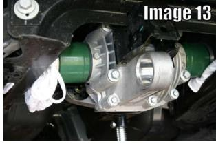
**NOTE:** If using BMR part number **BK046**, the Delrin bushing goes in the rear mount.
