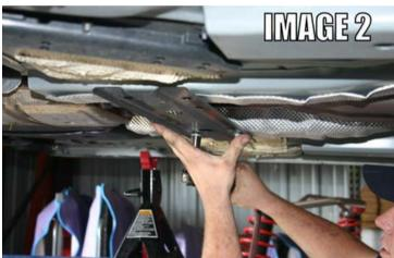
3. Using a 15mm socket, remove the driveshaft tunnel brace. See **Image 2**.
